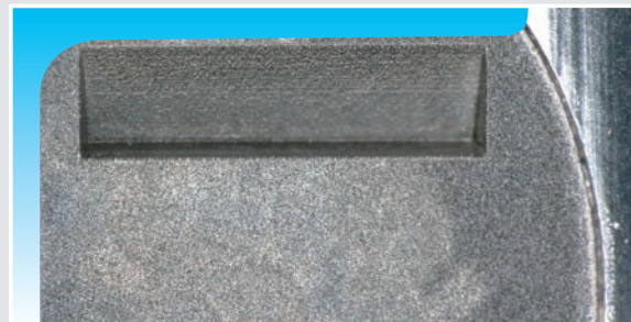
Enlarged view of breaker
